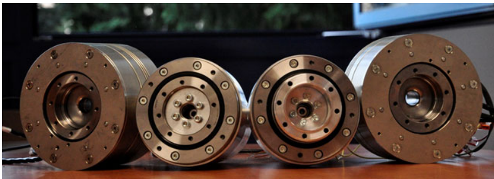
Fig. 4. Prototypes of modular flat- and cylindrical wheel strain wave drive systems
